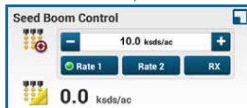
Seed Boom Rate Control – Utilizes the rates or prescription defined in the Pro 1200 Product Setup. UDW is active when Task Controller is selected.
