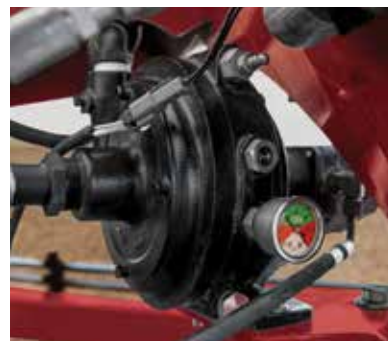
Barrier fluid sight glass and internal pump pressure gauge
