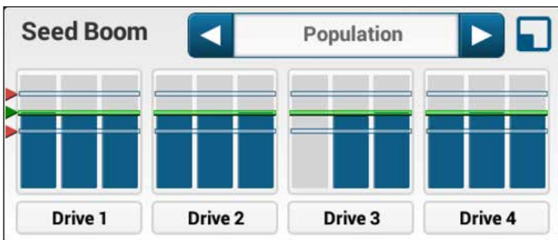
Seed Boom Bar Graph – Will display all ASI metrics related to seed monitoring. Select a drive or row for further performance detail.
