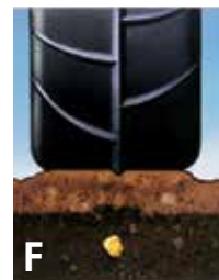
F Verify press wheel (if equipped) function ( F ).
